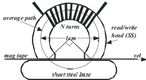
The system has been designed so that a drive current of 30mA is available to provide the field density of  $B = 1.3T$  needed to effectively magnetize the tape.
