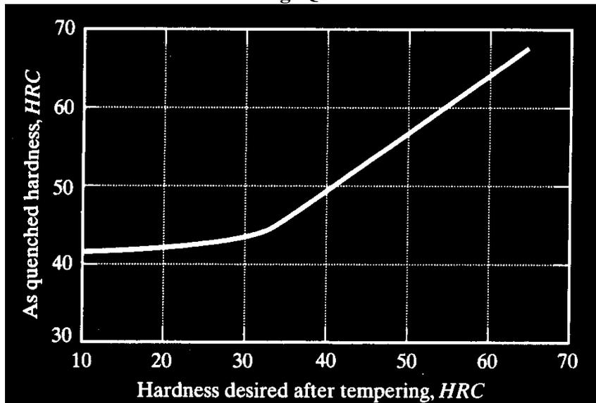
As-quenched hardness of steel as a function of the desired hardness (in HRC) after tempering.
