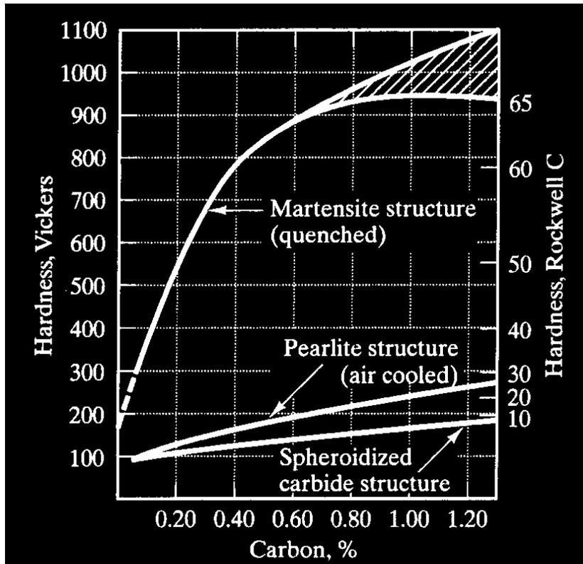
Hardness of ~100% as-quenched martensite, pearlite, and spheroidized microstructures as a function of carbon content
