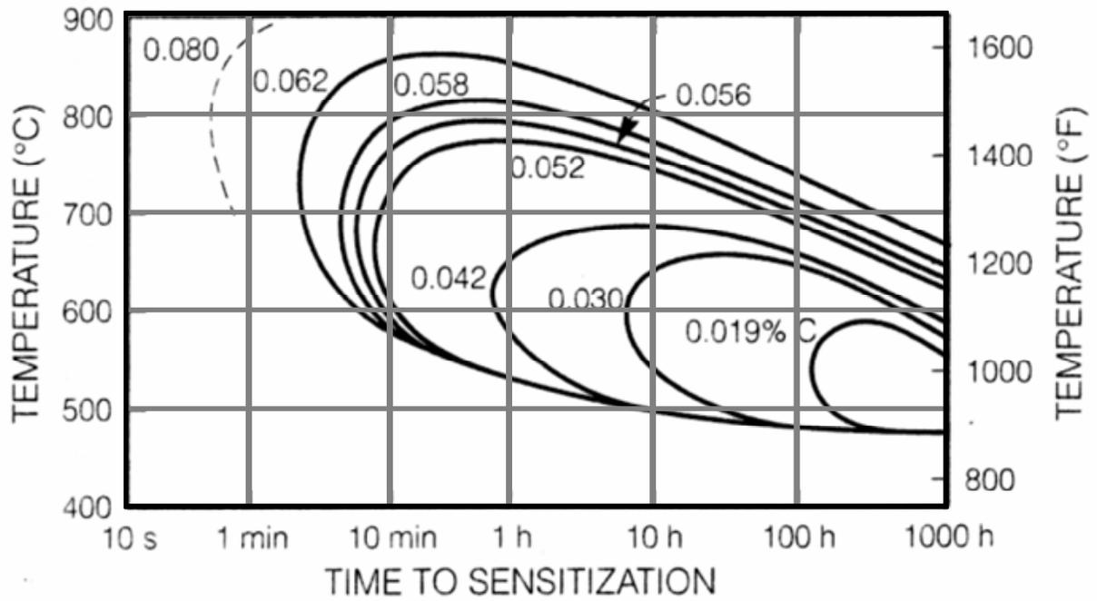
Figure Q4. Sensitization diagram for 18Cr-8Ni stainless steel of varying carbon content.
