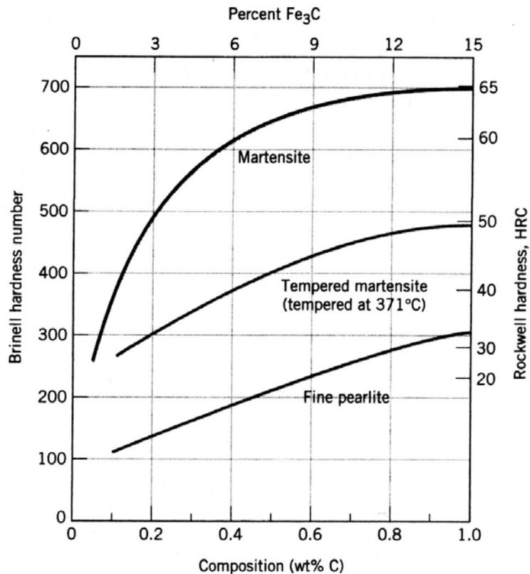
Hardness of martensite, tempered martensite and fine ferrite as a function of carbon content.
