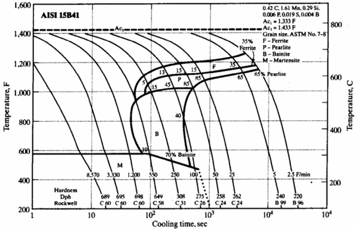
Figure Q6. CCT diagrams of AISI 1541 and 15B41 steels.
